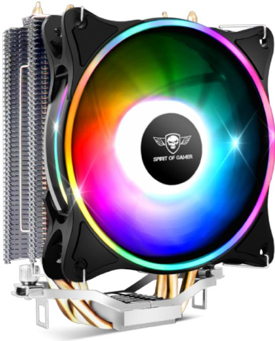
AIRCOOLER OFFRE UNE REFROIDISSEMENT HAUTE PERFORMANCE MAIS AUSSI UNE SOLUTION DE RÉTRO-ÉCLAIRAGE PERSONNALISABLE DU VENTILATEUR AIRFORCE 120 MM. EN EFFET, LA CONNECTIQUE RGB ADRESSABLE 3 PINS / 5V INCLUSE EST COMPATIBLE AVEC LES CARTES MÈRES : ASUS AURA SYNC, GIGABYTE RGB FUSION, MSI MYSTICLIGHT SYNC ET ASROCK POLYCHROME SYNC, UTILISEZ LE LOGICIEL DE VOTRE CARTE-MÈRE POUR PRENDRE LA MAIN SUR LES COULEURS DE VOTRE SETUP.
